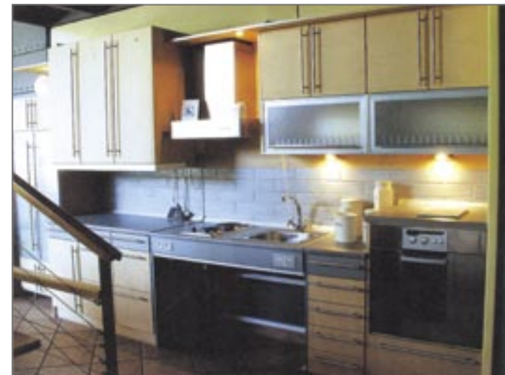
▲ Example of a kitchen designed for the needs of a wheelchair user. The cupboards over the counter are sliding, so that they can be adjusted in the proper position for the wheelchair user to reach.
